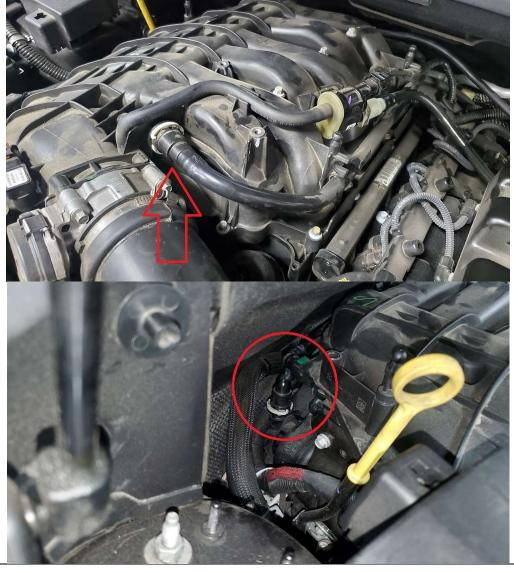
Page 1 of 4 1-27-23 Mount J&L bracket to J&L Oil Separator, align logos and use the supplied screws to secure the bracket.
